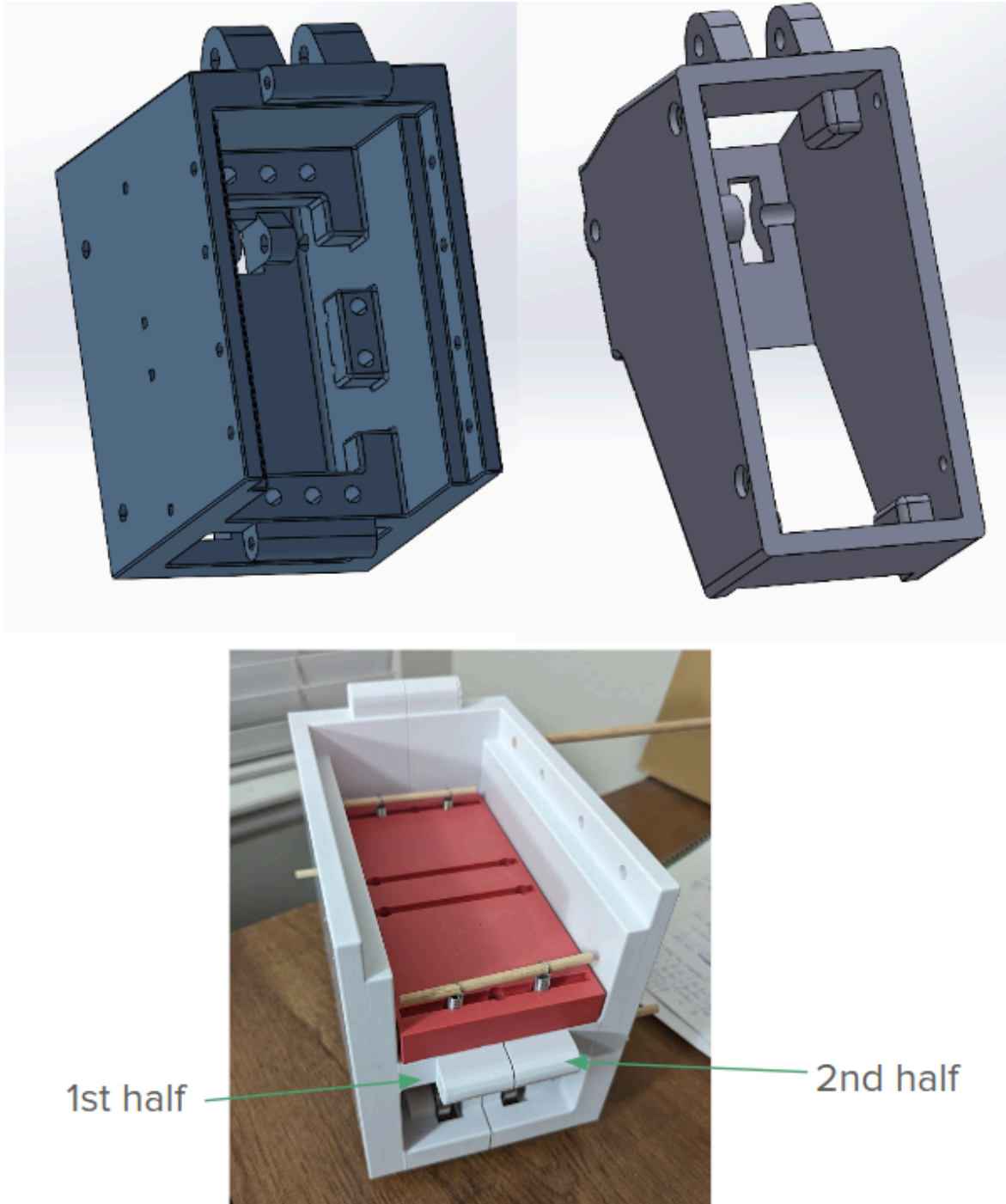
Figure 11 - Initial shell design (top left), final shell design (top right), and shell and slider prototype with tension springs and dowels (bottom)
